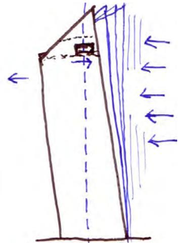
If the building sways left, the tuned mass damper moves to the right, straightening the building
